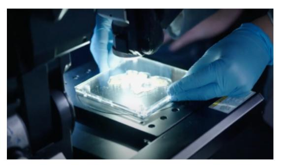
Thanks to a multi-spectral imaging system designed by NASA engineers, the scroll fragments are now able to be further documented & studied.
